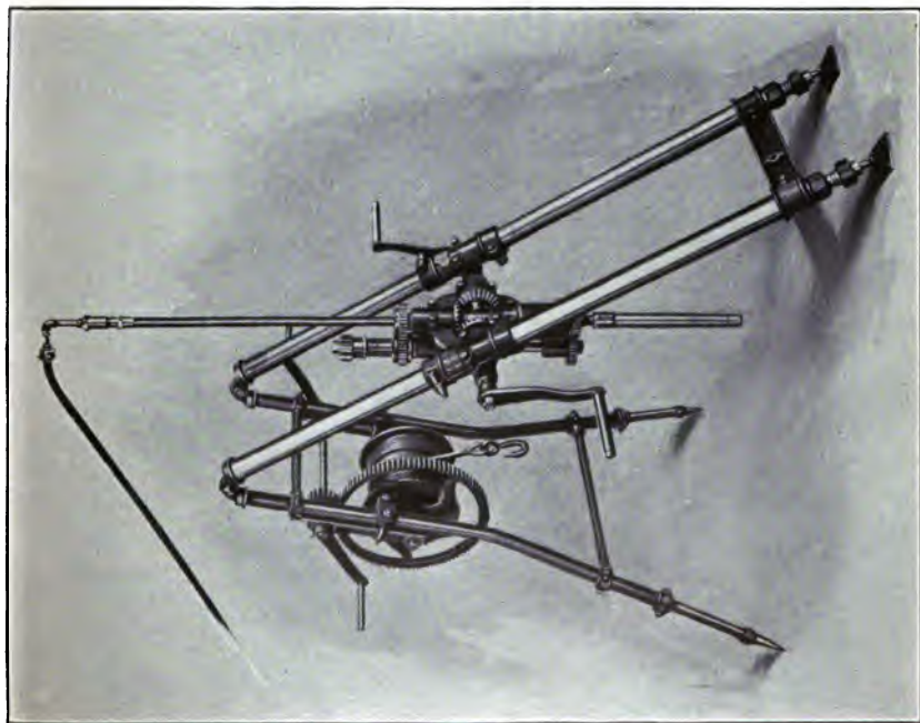
A. HAND-POWER DIAMOND DRILL, WITH FRICTION FEED.
